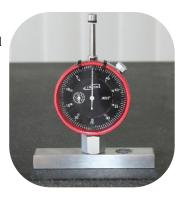
Zero setting when using extension rod and/or flat, needle, or spline point and with a pair of block, and on a flat surface.
