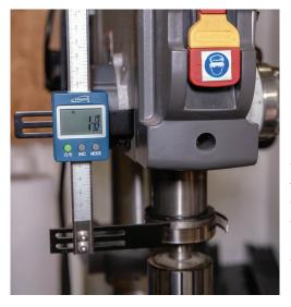
Improve the accuracy and precision of your hole drilling operations with the iGaging EZ-Depth gauge on your drill press. It is attached directly to the collar on the quill and to the side frame of the drill press. Zero the display with the drill bit in contact with the workpiece, then use the digital display to measure the drilled depth.
