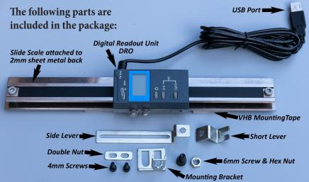
**Step 1:** Remove the existing red cursor and install the iGaging mounting bracket in the same machine screw holes using the bracket, double nut and 4mm screws.
